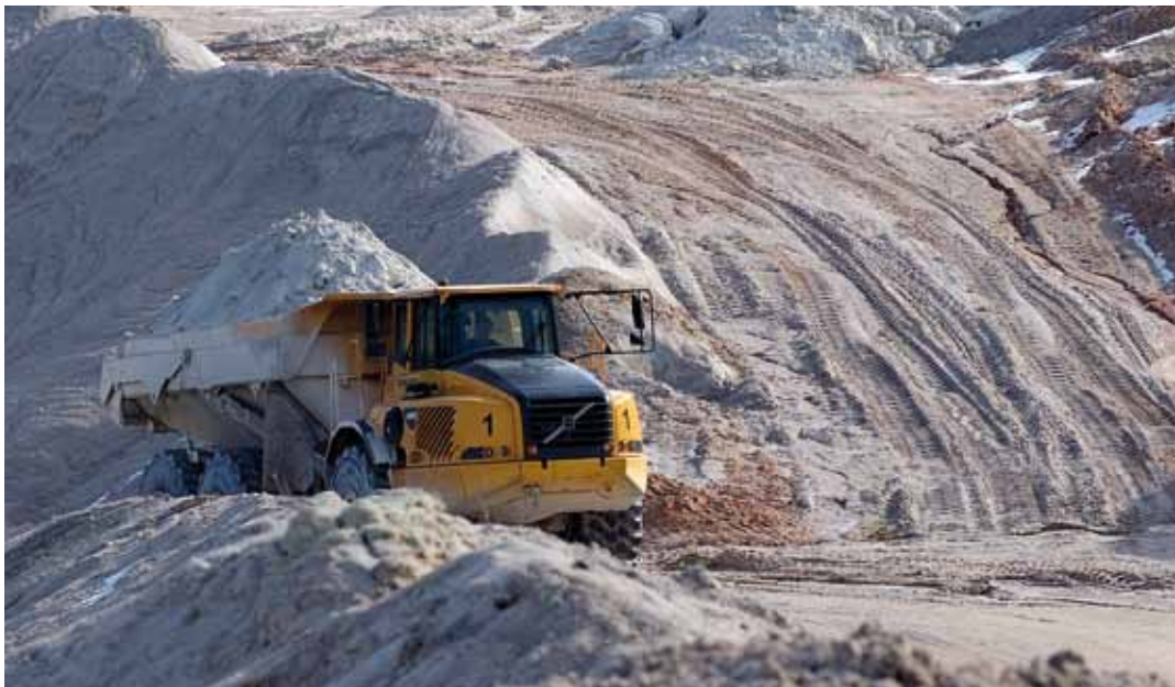
Selective extraction of soil containing kaolin at the Dorfner open-pit mine
