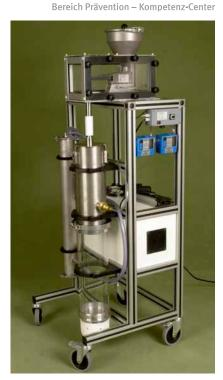
Continuous drop dust pipe apparatus at IGF used to measure dust
