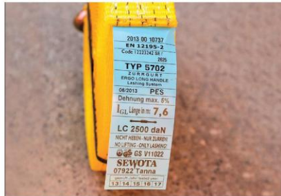
Suitable tension straps (2,500 daN) with blue label
